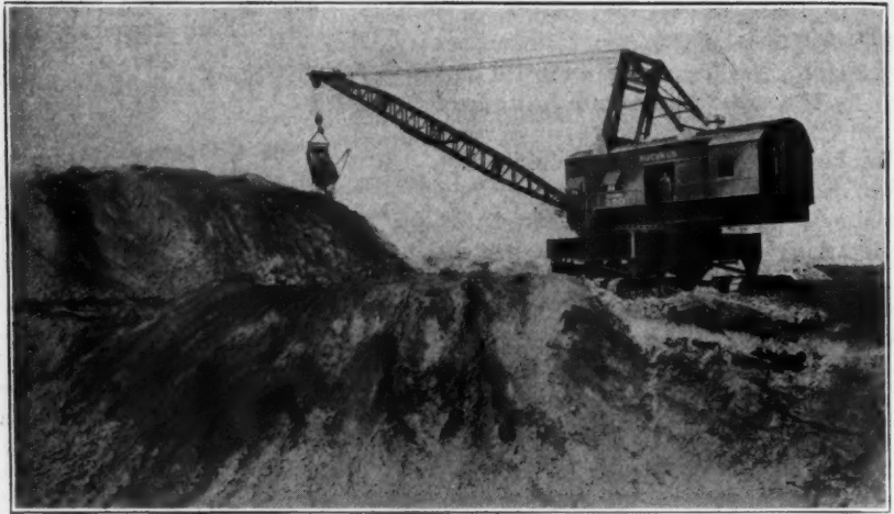
The 6-Yard Stripping Shovel Operating as a Dragline
